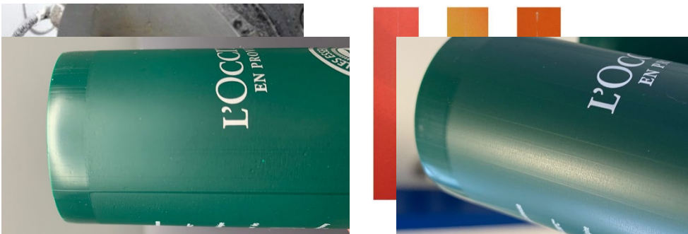
Figure 6: Scratching during extrusion
