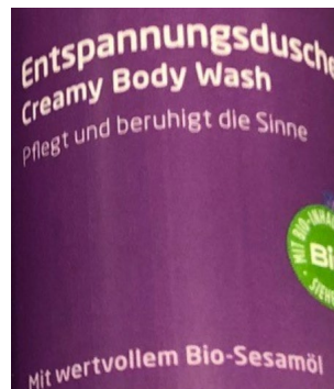
Figure 9: Solid printing with streaks
