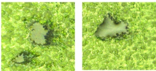
Figure 3: Damage to the printing plate under digital microscope (Zoom: 700x)
